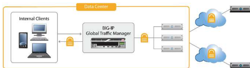
Figure 7: BIG-IP GTM is the DNS resolver responsible for requesting the additional DNSSEC records and doing the crypto calculations to validate that the DNS response is correctly signed.
