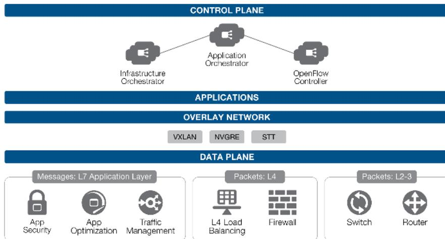
In a well-built L2-7 SDN architecture, all the components represented here are both necessary and complementary to one another.
